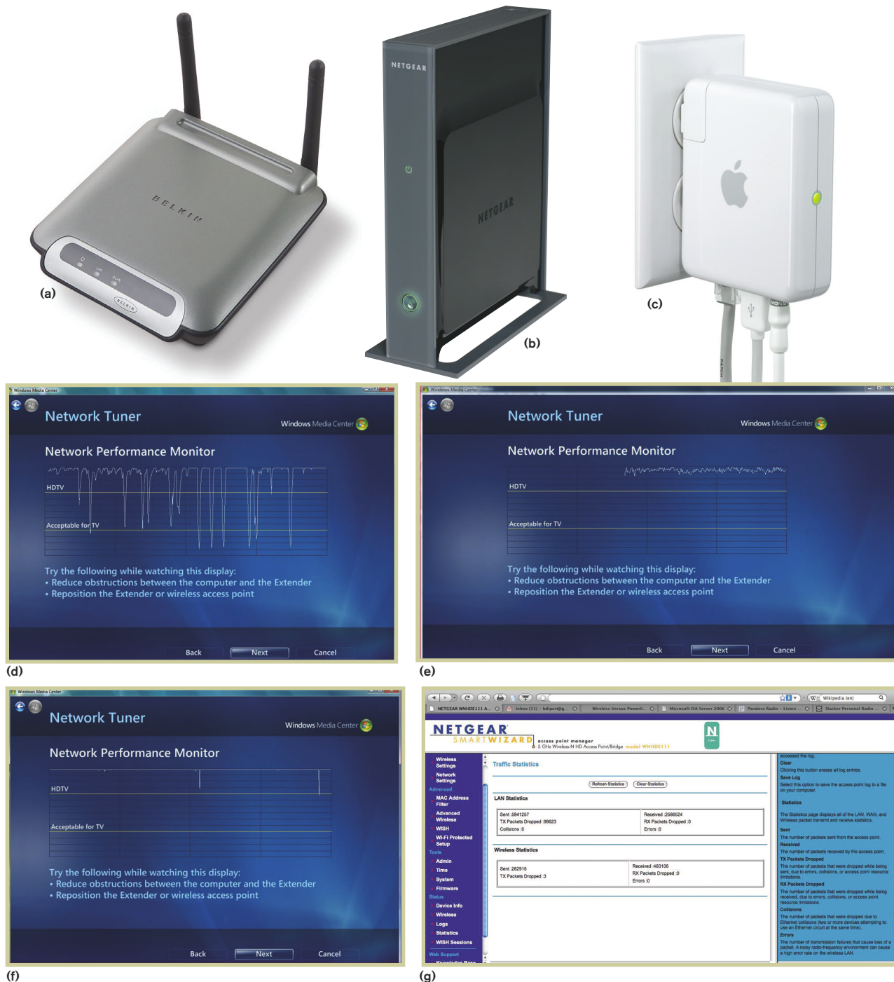
Figure 4 The Apple router's lack of simultaneous dual-band support necessitates the inclusion of an 802.11g access point for legacy LAN clients (a). Netgear's WNHD111 created a second 5-GHz bonded 802.11n channel (b), and I also used Apple's Airport Express N access point during debugging (c). Regardless of their frequency bands, the simultaneous operation of two 802.11n signals resulted in quality-degrading packet-loss glitches (d), which did not occur when part of the source-to-destination span relied on HomePlug AV (e) or Category 5e wired Ethernet (f). Diagnostics reports point to the router's switch as the culprit (g).
